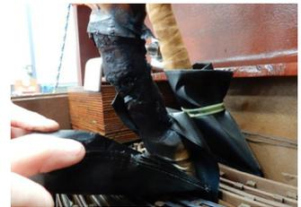
Winding connection leads with severe carbonisation (burning) of paper insulation.
