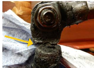
Burnt winding connection lead with a large crack (yellow arrow)
