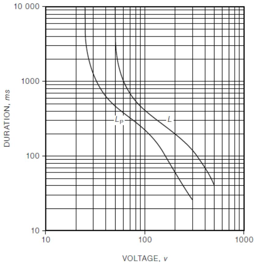
*L* for normal conditions touch voltage limit 50 V
