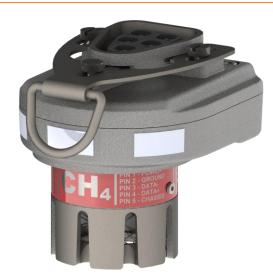
gas reduces the amount of infrared energy reaching the detector. This difference in infrared energy with and without gas is used to measure the amount of gas present, and is converted to a digital value by the integrated sensor electronics. The sensor conditioning is fully self-contained and stores all necessary compensating and calibration information to provide a linear temperature compensated output.
