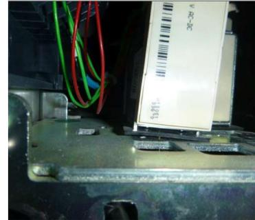
Fig. 4 MN coil found out of position (with vibration pad underneath)
