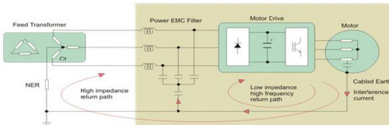
Figure 2: alternate earth leakage current path via the power EMC filter associated with the VSD
