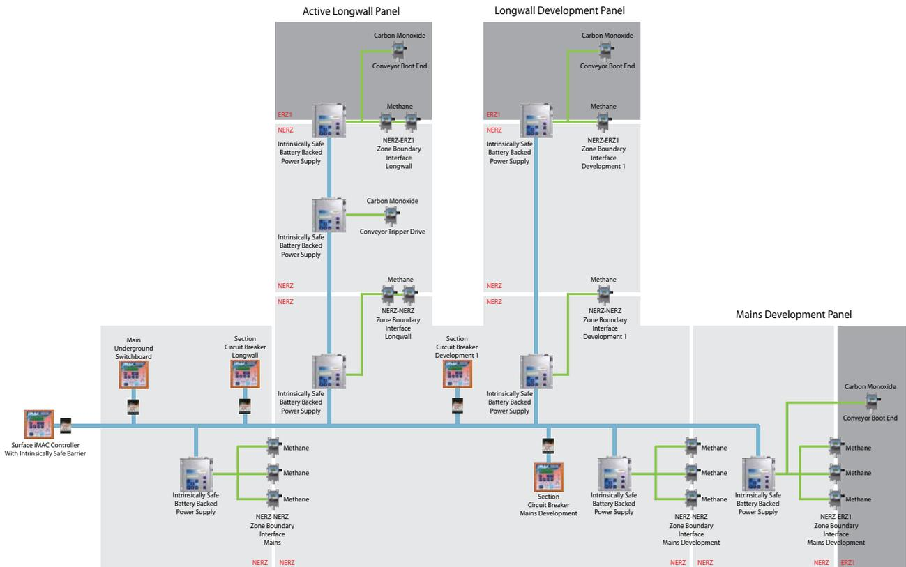
Figure 2: An example of the NERZ - NERZ and NERZ - ERZ system architecture
