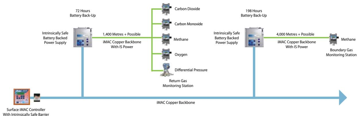
Figure 1: Examples of Intrinsically Safe power supply deployment
