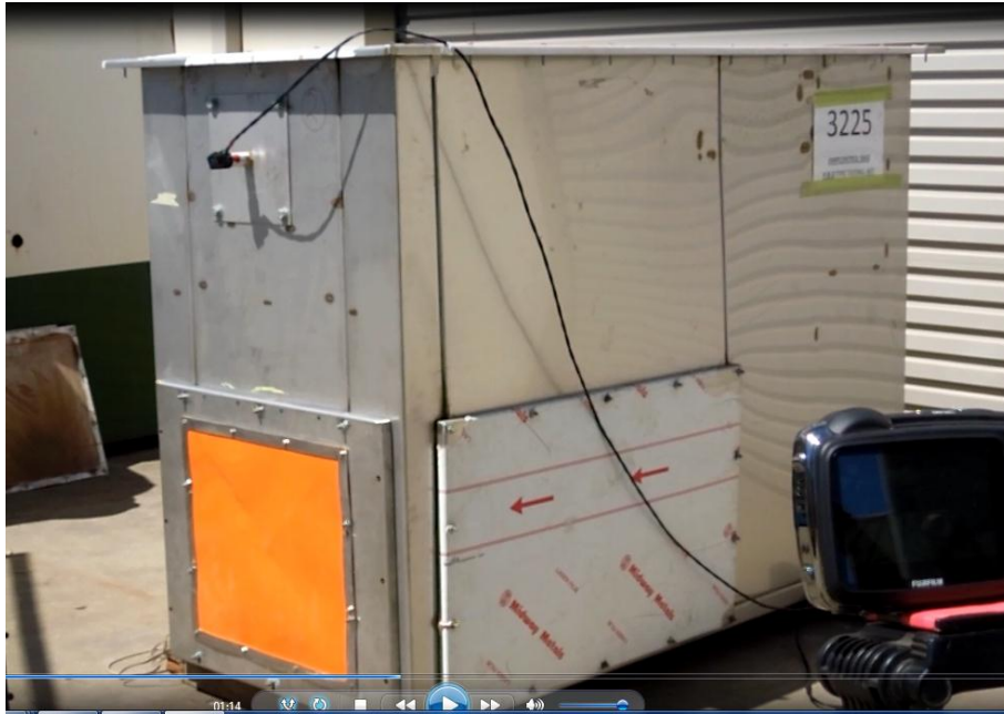
Figure 3: Arc fault vent fitted to IP55 enclosure.
