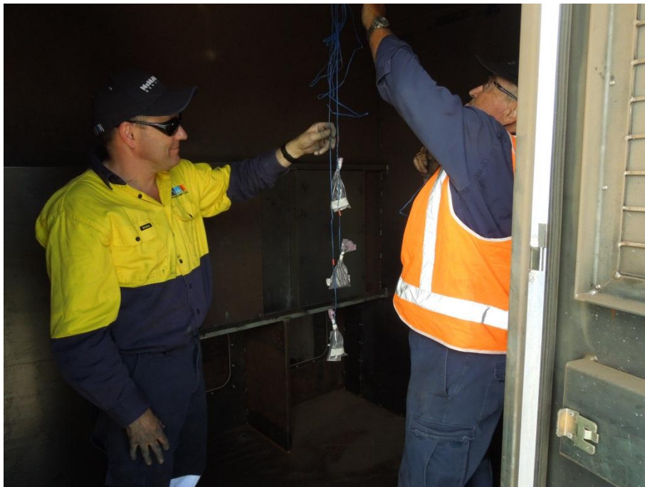
Figure 2: Energetic materials used to generate pressure rise simulating nominated arc fault level.
