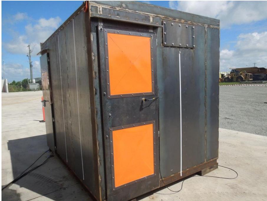
Figure 11: Switchroom from Figure 5 after simulated 30 kA test. The upper vent has ruptured, and then closed once pressure released.
